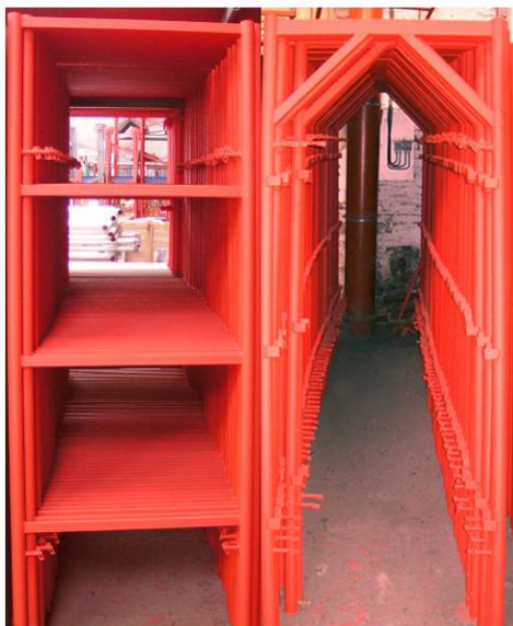
Figure 20: Example of scaffolding frame [Ref.21]
